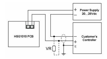
VR - for achieving a DC voltage signal, as alternative to the standard 4...20mA signal, connect a fixed resistance across the 'customer' input:
